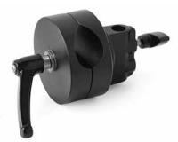
for pipes with diameters of 1.2" (30 mm) and 1.4" (35 mm). Locking takes place with an anti-friction disc, and a thrust bearing assisted by a robust knob. The body has a housing for a .6" (16 mm) diameter pin, locked by the relative knob. All components are produced in die-cast aluminum painted black. Weight 2lbs (0.9 kg).
