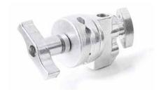
flanges (diameter 2.6" or 65 mm) have housings for pipes with diameters of .4" (10 mm), .5" (12 mm), and .6" (16 mm). Locking takes place with an anti-friction disc and with a thrust bearing supported by a robust knob. The body is fixed on a .6" (16 mm) diameter pin and locked by the relative knob. All components are produced in die-cast aluminum, polished or painted black. Weight 1.3lbs (0.6 kg).
