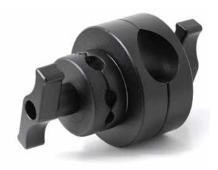
of 3.9" (100 mm) have housings for pipes with a diameter of 1.2" (30 mm) and 1.4" (35 mm). In addition, the two small round flanges with a diameter of 2.5" (65 mm) have housings with diameters of .4" (10 mm), .5" (12 mm), and .6" (16 mm). Locking takes place with an anti-friction disc and with a thrust bearing supported by two robust knobs. All components are produced in die-cast aluminum painted black. Weight 2lbs (0.9 kg).
